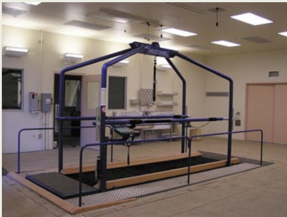
The new Equine Athletic Performance Laboratory will offer two Swiss Mustang 2200 motorized equine treadmills for evaluating performance problems and implementing new therapeutic approaches for treating them. These treadmills are among the most sophisticated in the world today, capable of reaching racing speeds of over 37 mph.
